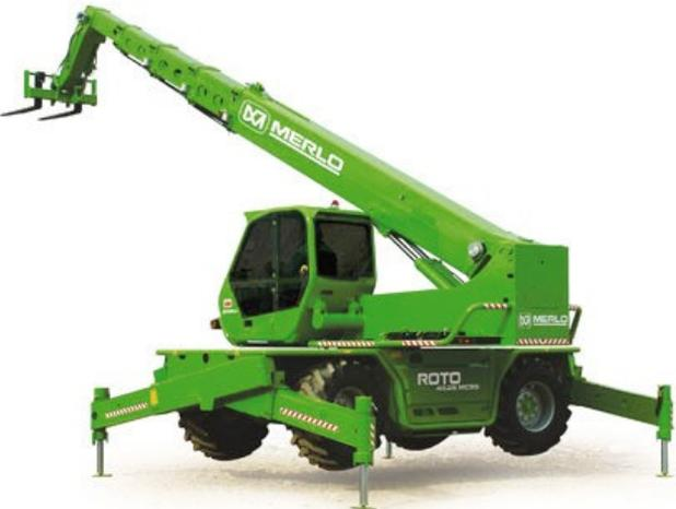
A green Merlo 38.16 Roto telescopic loader with a long-reach boom and a pallet fork attachment. The machine is shown from a side profile, facing left. It has a more complex design with a long telescopic boom and a stabilizer system with outriggers. The Merlo logo and 'ROTO' are visible on the machine.
